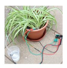
• Example code can be found on our website at the following link <u>https://sciencescope.uk/product/microbit-plant-watering-system/</u>. This code uses the micro:bit soil moisture sensor and the micro:bit water pump to maintain a healthy soil moisture level of a plant. Use the buttons to control the water pump a view the soil moisture level.
